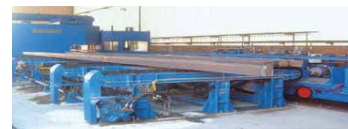
Billet conditioning with grinding machine
