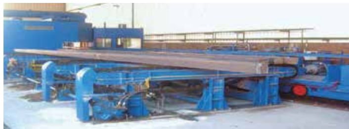
Billet conditioning with grinding machine
